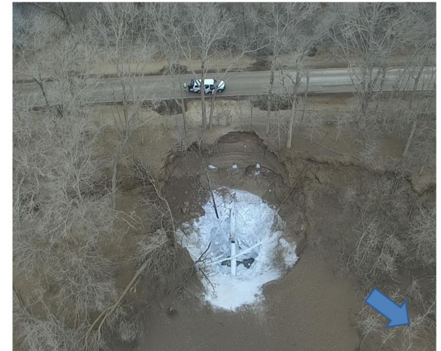
Figure 2: Vehicle is Parked on HWY 433 - The White is Ice Generated by the Release of CO 2 - The Blue Arrow Points North (Aerial Drone Photograph Courtesy of the Mississippi Emergency Management Agency)
