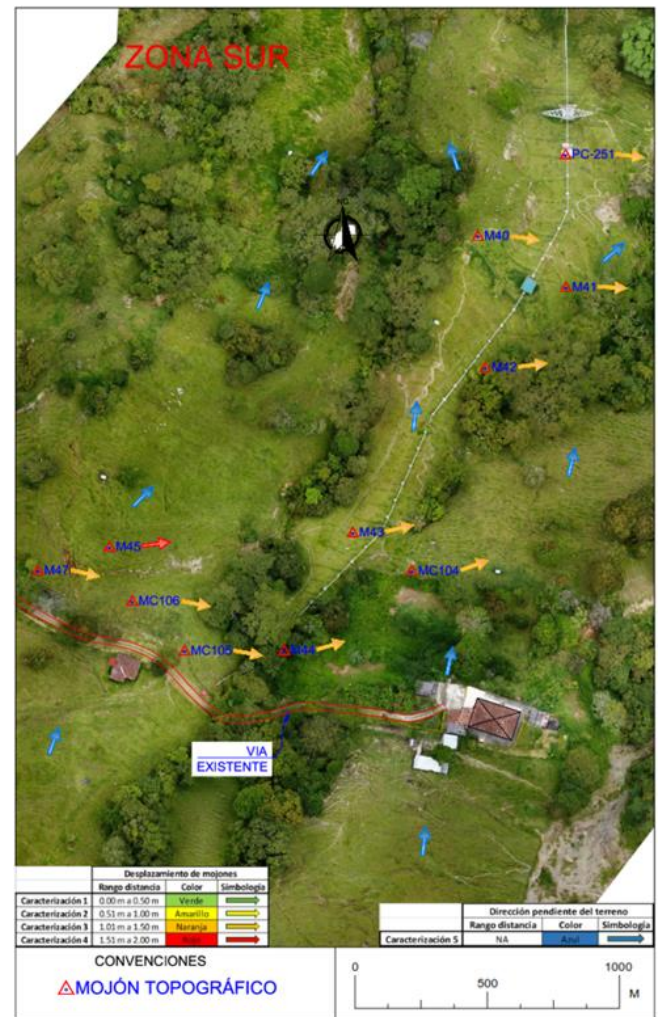
FIGURA 5: TOPOGRAPHIC DISPLACEMENT VECTORS ON THE SOUTHERN SLOPE
