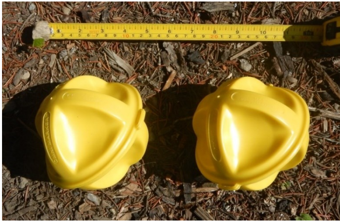
FIGURE 5: MARKER BALLS FOR MONITORING NEAR SURFACE GROUND MOVEMENTS.
